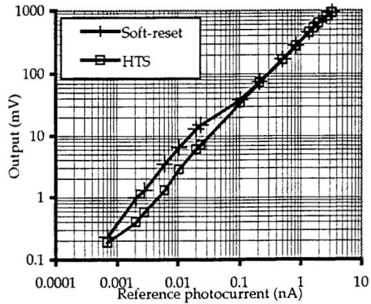
Figure 11: Measured response for soft and HTS reset
