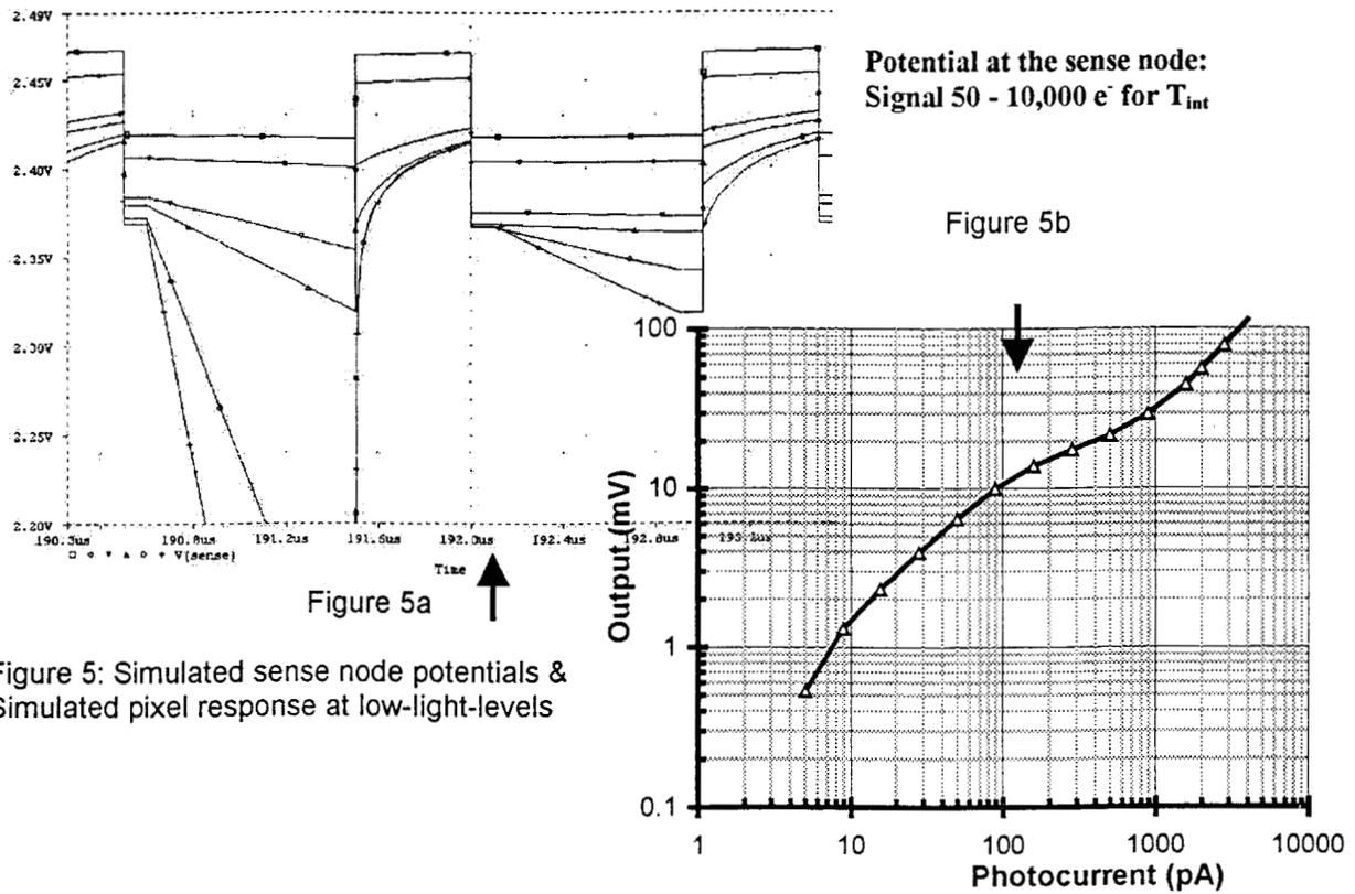
Figure 5: Simulated sense node potentials & Simulated pixel response at low-light-levels
