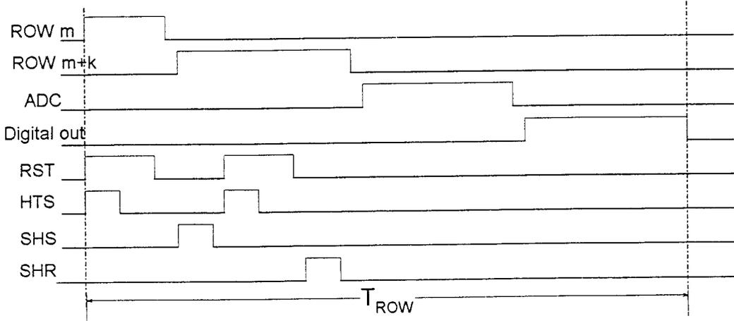
Figure 3: Pixel and row timing diagram
