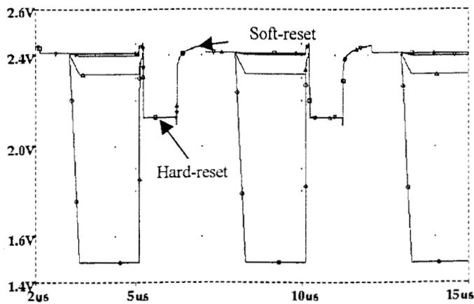
Figure 6: Simulated sense node potentials for HTS reset scheme
