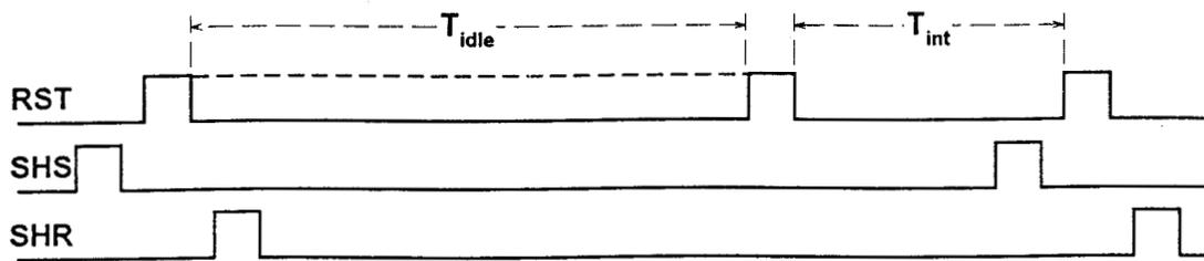
Figure 4: Timing diagram for still or high-speed video mode imaging (No HTS pulse is used)
