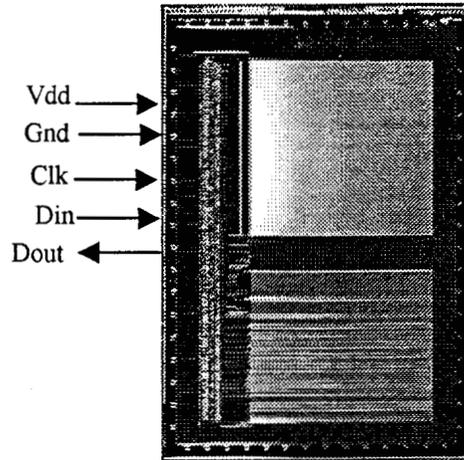
Figure 9: Microphotograph of the one-chip digital imager
