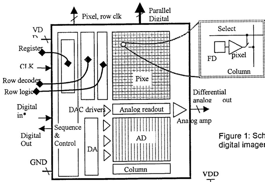
Figure 1: Schematic of the one-chip digital imager
