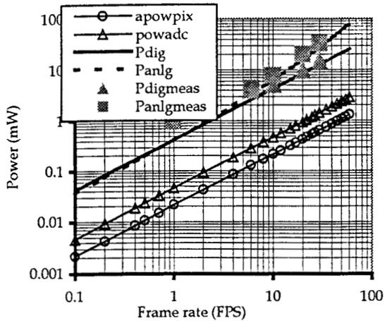
Figure 8: Power dissipation and its components as function of frame rate
