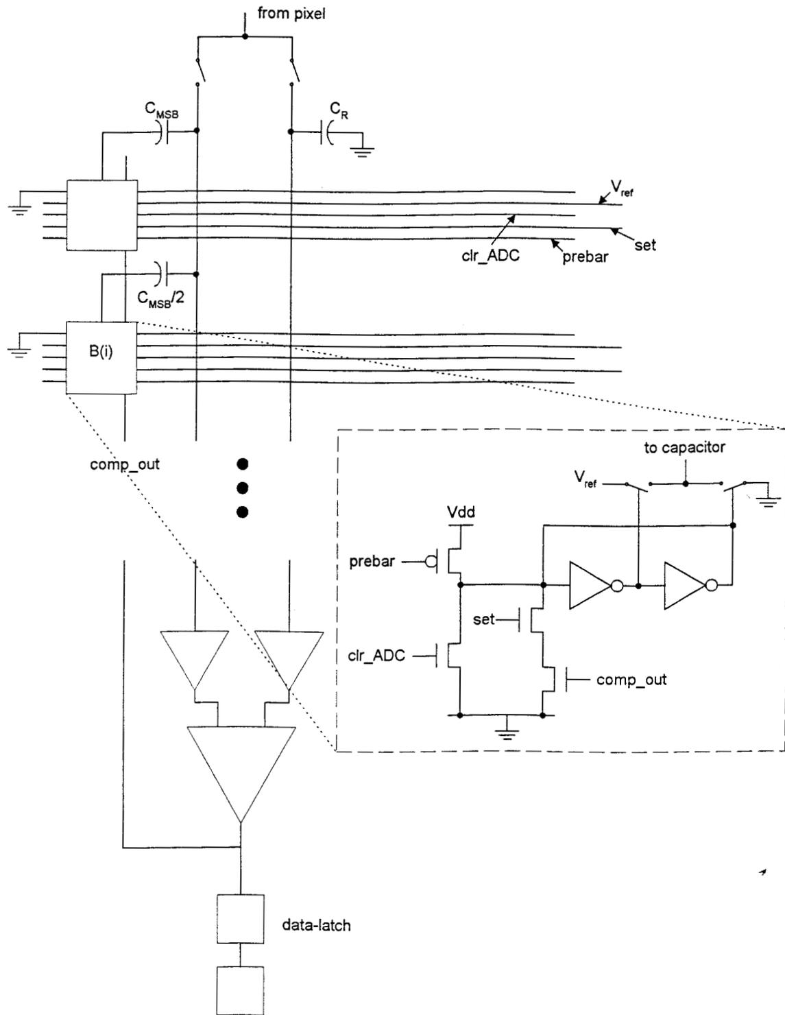
Figure 7: All-capacitor successive-approximation ADC implementation with the bit-cell circuit
