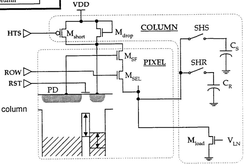
Figure 2: Schematic of the pixel and column signal chain of the digital imager
