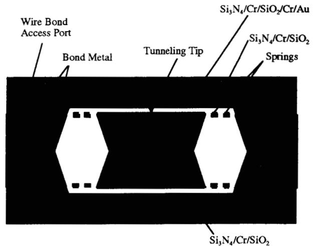
Figure. 1 Accelerometer Cross Section
