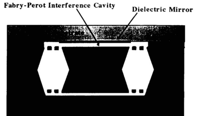
Figure 5 Fabry-Perot Filter Cross Section
