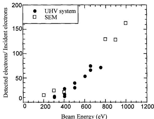
Figure 5 Ratio of detected electrons to incident electrons as a function of energy. The response of the CCD increases with increasing energy as result of multiple electron-hole pair generation.
