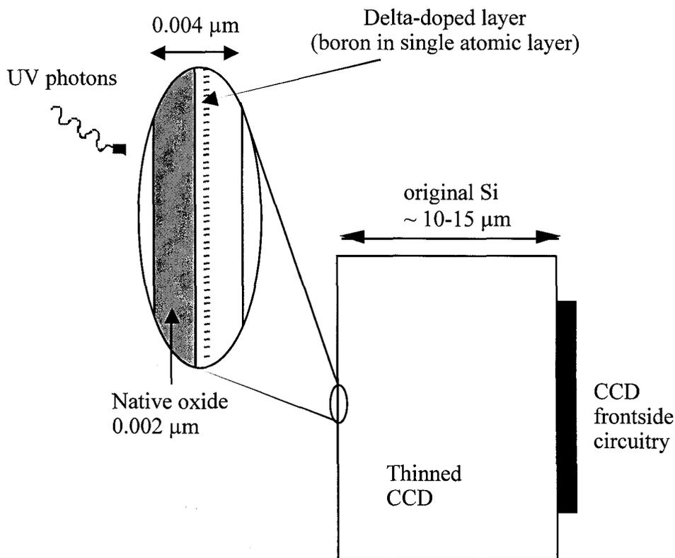
**Figure 1.** Cross section schematic of a delta-doped CCD. The epitaxially-grown delta-doped layer on the back surface of a thinned CCD places a high density of boron atoms approximately 0.5 nm below the silicon epilayer surface and protected by an oxide overlayer.
