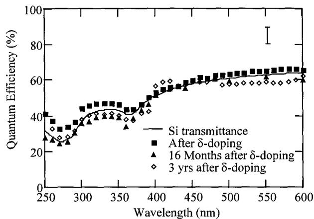
Figure 4. QE measured over a three-year period on the same delta-doped 512-by-512-pixel Reticon CCD. The CCD was stored unprotected in a laboratory environment. The error bars represent the accuracy ( $\pm 5\%$ ) of the measurement systems used.
