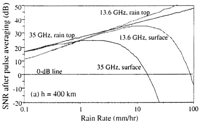
Figure 1. Expected signal-to-noise ratios for the PR-2 system at 400-km altitude.
