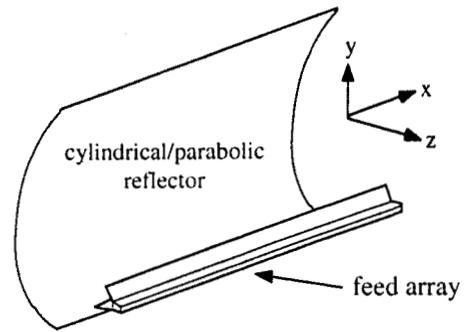
Figure 2. Configuration of a cylindrical/parabolic reflector illuminated by a linear array.
