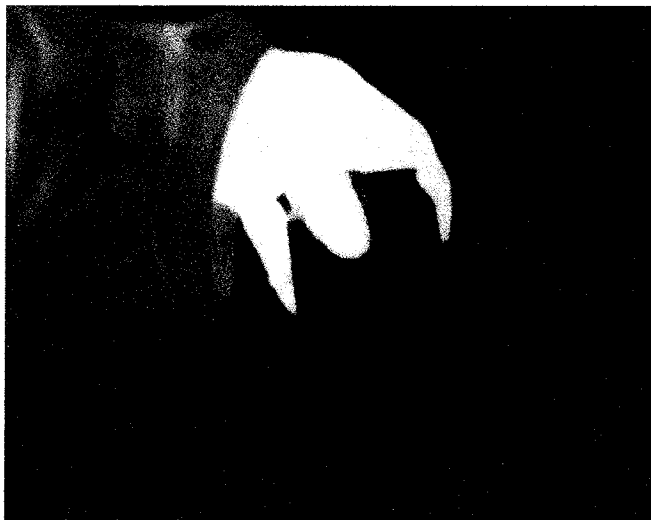
Fig. 11. This picture shows a frame of video image taken with this 10-15.4 mm 640x512 broadband QWIP imager. This image shows the liquid level of the soda can and some finger prints on the can.
